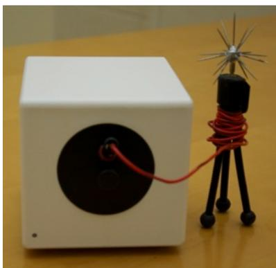
2. Next, insert the Titanium Cylinder Insert into the lens window on the front of the device. Be sure to first remove the Finger Insert from the lens window. To remove the Titanium Cylinder Insert, gently press down on the bottom, outer edge of the Finger Insert and gently pull outward, taking care not to scratch the lens.
